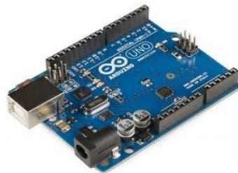
Gambar 7. Board Arduino Uno
