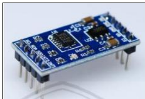
Gambar 7. Sensor Accelerometer ADXL345 Sumber: Devices, 2021
