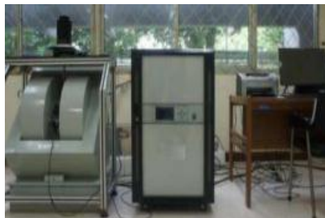
Gambar 26. Alat Uji Vibrating Sample Magnetometer LIPI Fisika. (Emma Rosinta, 2017)
