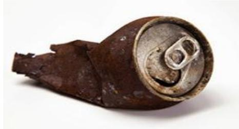
Gambar 1. *Uniform/General Corrosion*
