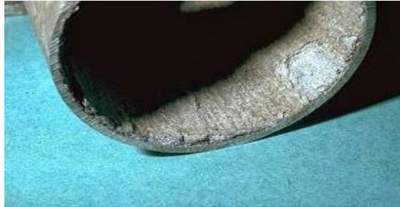
Gambar 6. *Intergranular corrosion*
