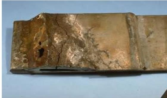
Gambar 7. *Stress corrosion cracking* (SCC)
