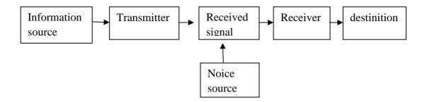
The figure above can be illustrated as communication is begun from deciding the information source that wants to be sent. This message is then changed by the transmitter to into a signal which is sent through the channel to the receiver. For a telephone, the channel is a wire and the signal is the electric current in it. While in conversation, the mouth is the transmitter, the signal is the sound waves, which pass through the channel of the air, and the listener's ear is the receiver.
