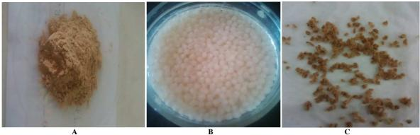
Figure2: Non immobilized (A), gel(B) and drybead(C) bio-sorbent.
