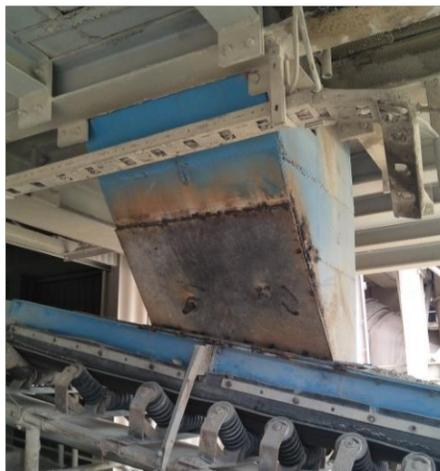
**Gambar 2.14** *Discharge Chute*
