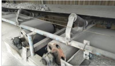
**Gambar 2.8** *Bend Pulley*
