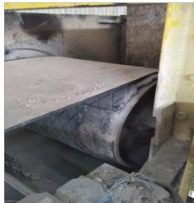
**Gambar 2.6** *Drive Pulley*
