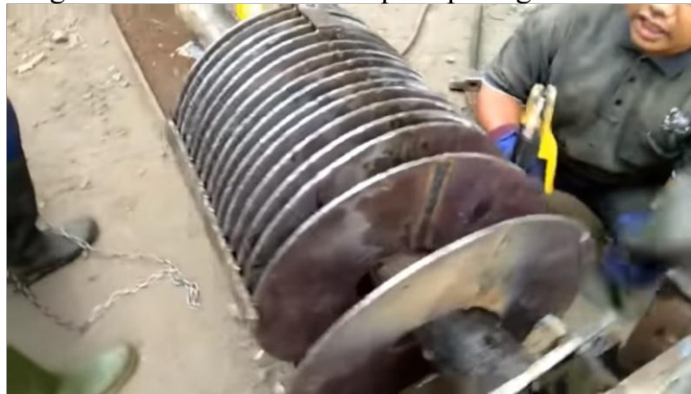
Gambar 4.5. pengelasan daun screw conveyer ke besi poros
