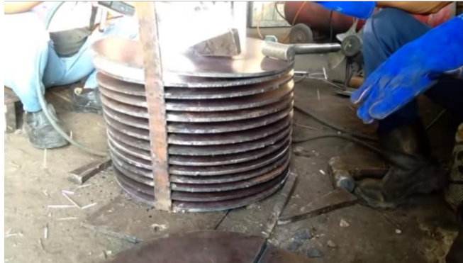
Gambar 4.4 penggabungan daun screw conveyer
