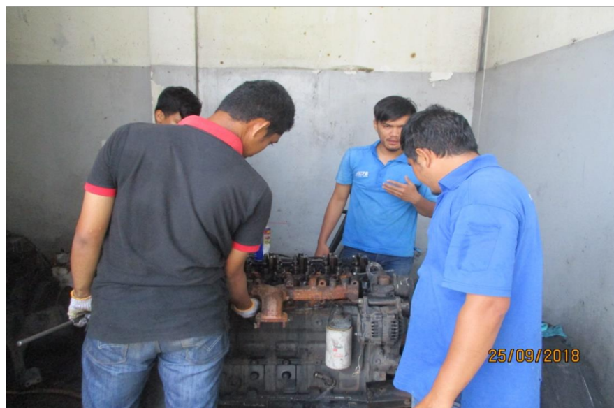
Gambar 10. Proses Disassembly Engine 6 BTA 5.9 Unit Kawasaki Wheel Louder 60 Z IV-2 (Sumber : Dokumentasi Perusahaan)
