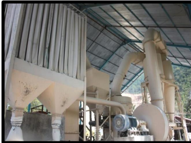
**Gambar 1.5 Mesin MTM (Medium Speed Trapezium Mill)**
