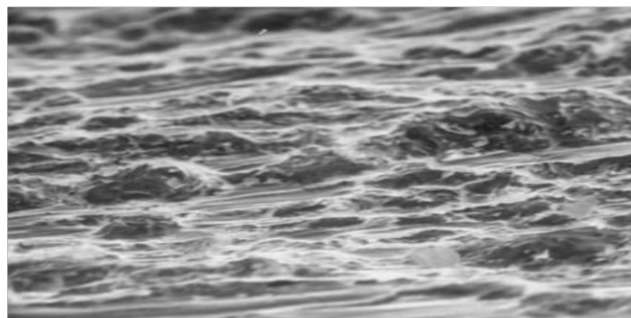
2.15 Permukaan patah shaft roda coil car
