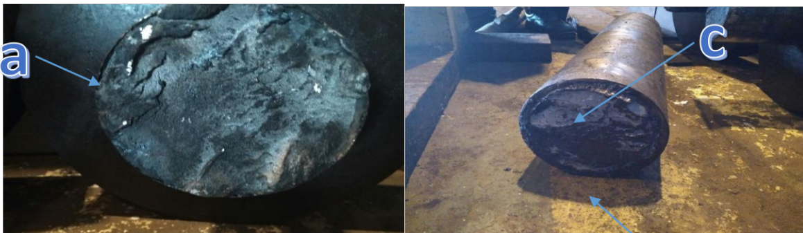
2.14 Permukaan patah shaft roda coil car b
