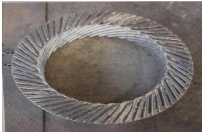
Gambar 28. *Stator Blend Cutter*
