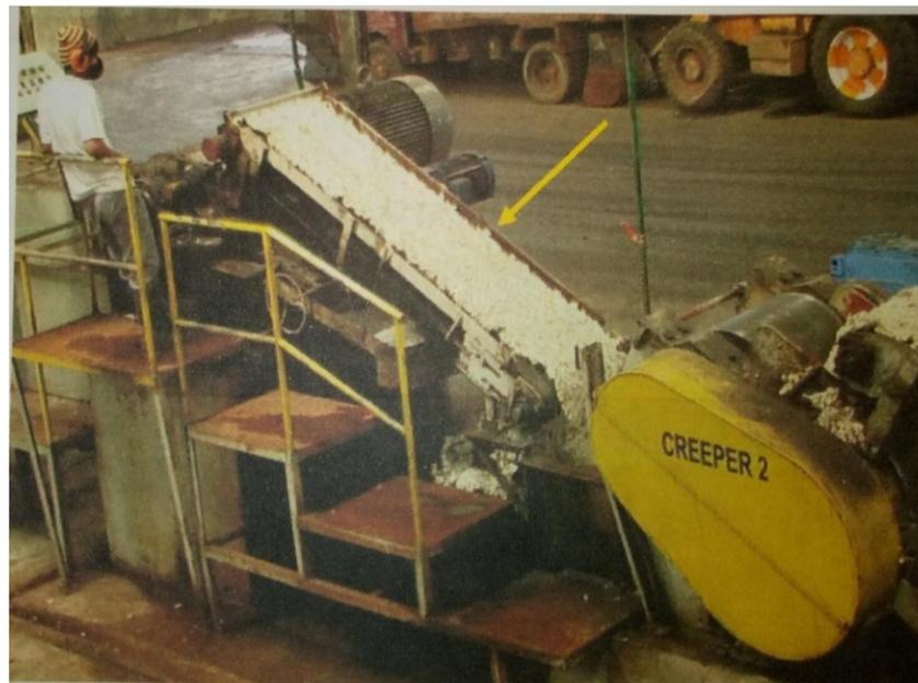
Gambar 32. *Belt Conveyor Creeper-Shredder*
