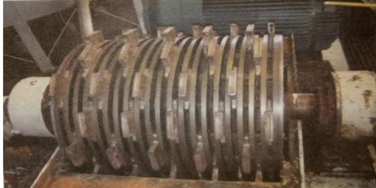
Gambar 23. Rotor *Hammermill*
