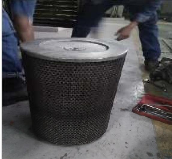
Gambar 4.9 *Air Filter Cartridge*
