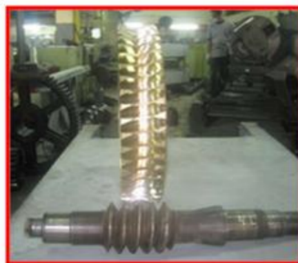
Gambar .2.2 Foto Kerusakan Gear dan Bearing Opening Gate Intak
