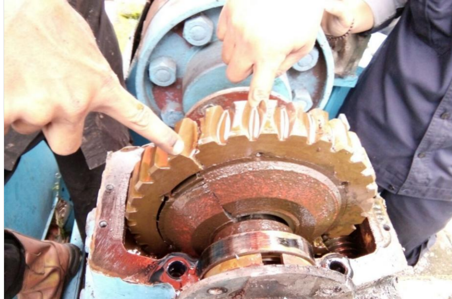
Gambar .2.2 Foto Kerusakan Gear dan Bearing Opening Gate Intak
