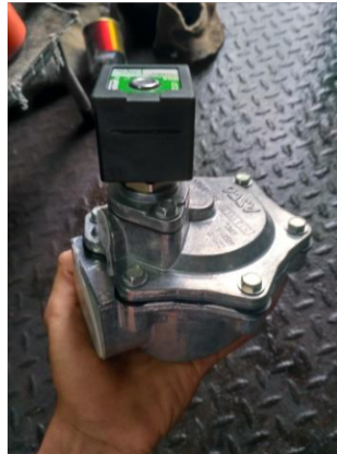
Gambar 4.8 Solenoid Valve (Sumber : Area Gudang Jet Pulse Filter)
