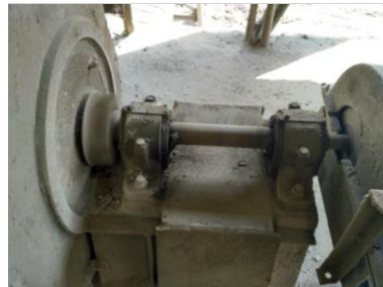
Gambar 4.4 Bearing dan Poros (Sumber: Bagian Area Jet Pulse filter, air sluice, apron conveyor, Indarung V PT. Semen Padang)
