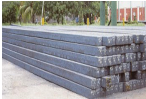
Gambar 2.7 Hasil Proses produksi billet steel plant
