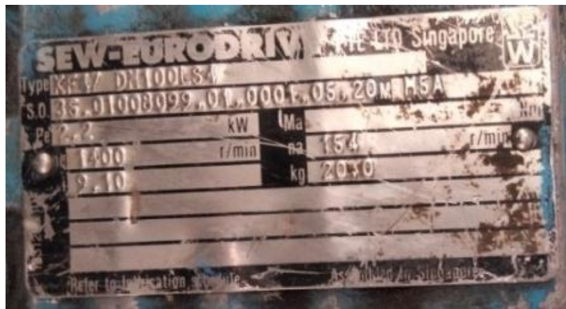
Gambar 4.7 Name Plate Motor (U01)
