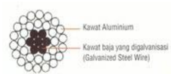
Gambar 15. Kawat ACSR ( Aluminium Conductor Steel Reinforced )
