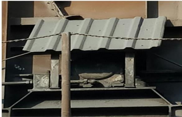
Gambar 4.6 Atap Pelindung Housing Bearing
