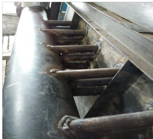
Gambar 35. Welding Pipa Steam Water Tube Ø 50.8 x 5 mm x 2500 mm Sumber . PT Jaya Sentrikon Indonesia
