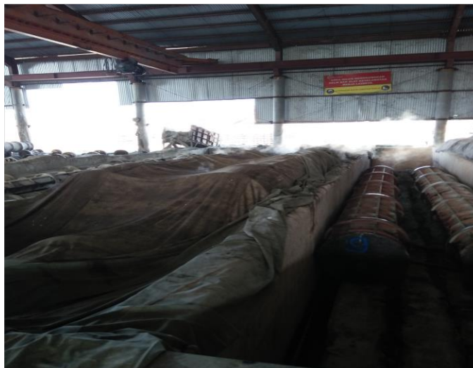
Gambar 15. Proses steam ( pengeringan ) Sumber . PT Jaya Sentrikon Indonesia
