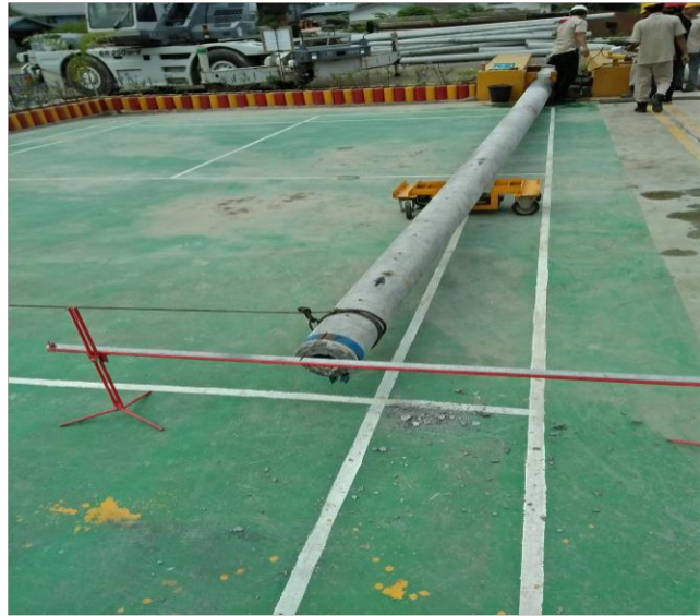
Gambar 17. Bending test ( tiang listrik ) Sumber . PT Jaya Sentrikon Indonesia
