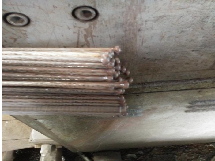
Gambar 8. Steel Bar (Heading) Sumber : PT . Jaya Sentrikon Indonesia
