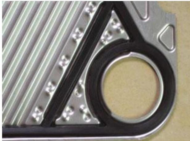
Gambar 2.2 Plat Heat Exchanger Tipe Glue
