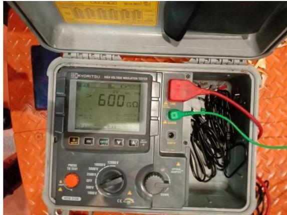
**Gambar 2. 5 Insulation Tester**
