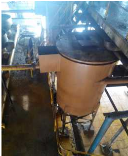
Gambar 9. Sand Trap Tank
