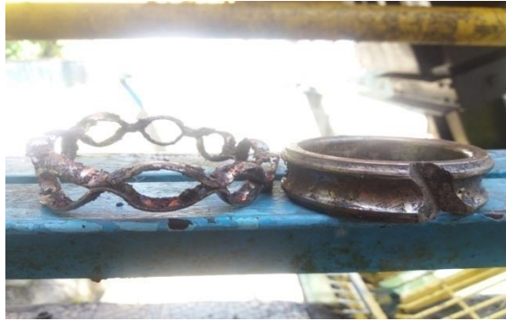
Gambar 4.5 Kerusakan Deep Groove Ball Bearing
