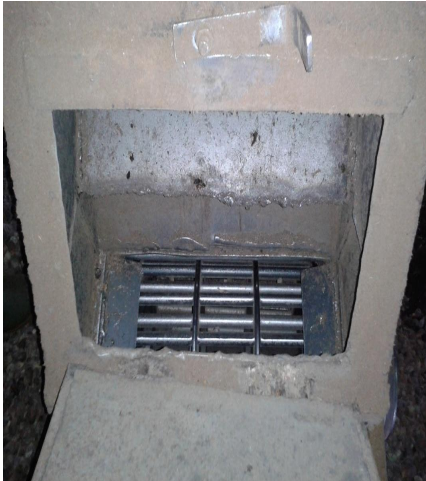
Gambar 10: Rotor ripple mill kehausan
