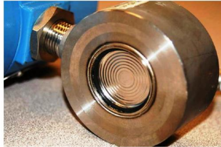
Gambar 18. Sensor Differential Pressure Transmitter (sumber : https://kontrolinstrumentasi.blogspot.com )
