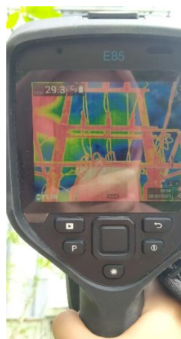
Gambar 8. Pengukuran suhu jumperan trafo
