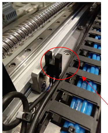
Gambar 3.58 Permasalahan Sensor Photo Eletric
