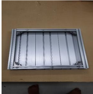
Gambar 3.37 Base Panel Sudah Ter-assembly
