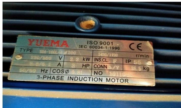
Gambar 10. Name Plat Motor 3 HP
