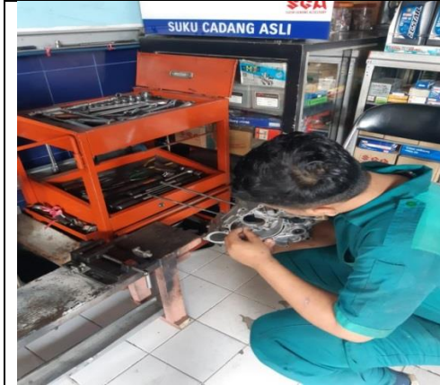
Gambar 7 Pengecekan Kebocoran Crankcase Shogun 110
