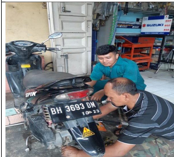
Gambar 5 Proses Pergantian Kampas Rem Spin
