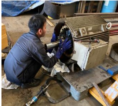
Gambar 2. 33 Proses Penggantian Bearing
