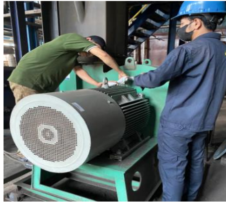
Gambar 2. 28 Proses Pemberian Grease motor
