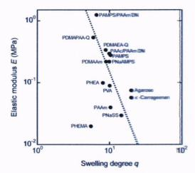
Figure 4. The relationship between the elastic modifiles ((E)) and the swelling degree (q) of the hydrogels. The busiken line indicates the scaling relationship of  $E-q^{-3}$ .
