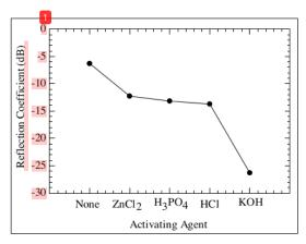
Fig. 4. The maximum reflection coefficient of the activated carbon for several activating agents at a material thickness of 10mm, concentration of 1M and frequency center of 8 GHz.
