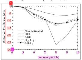
Fig. 3. Measured reflection coefficient of the carbon and the activated carbon with several types of activating agents (HCL, KOH, H<sub>3</sub>PO<sub>4</sub>, and ZnCL<sub>2</sub>) at a material thickness of 10mm.
