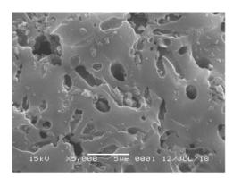
Fig. 10. The scanning electron microscopy (SEM) image of activated carbon of the palm shell with a magnification of 5000x for 1M KOH concentration
