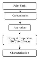
Fig. 1. Step by step of the active carbon production of the palm shell
