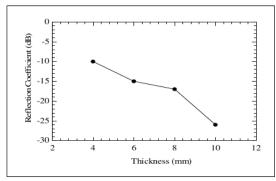
Fig. 8. Dependency between absorption and material thickness of the activated carbon at frequency center of 8 GHz and activating agent of KOH 1M
