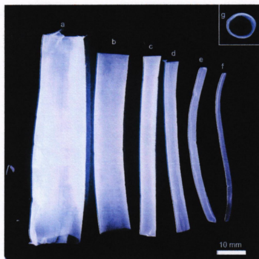
Fig. 3. The BC-TS gels cultured in the silicone tubes of various inner diameters: (a–f) lateral view of BC-TS with an outer diameter of 20, 10, 5, 4, 3, and 1 mm, respectively, and (g) top view of BC-TS with an outer diameter of 10 mm.
