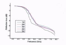
Figure 2. Reflection coefficient plotted as a function of frequency for variation of HCL activator concentration at thickness 8mm.
