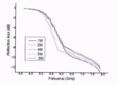
Figure 3. Reflection coefficient plotted as a function of frequency for variation of HCL activator concentration at thickness 10 mm.
