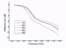
Figure 1. Reflection coefficient plotted as a function of frequency for variation of HCL activator concentration at thickness 6mm.
