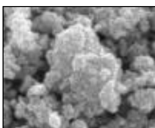
Figure 7. Agglomeration Occurring On Hausmannite Nanoparticles
