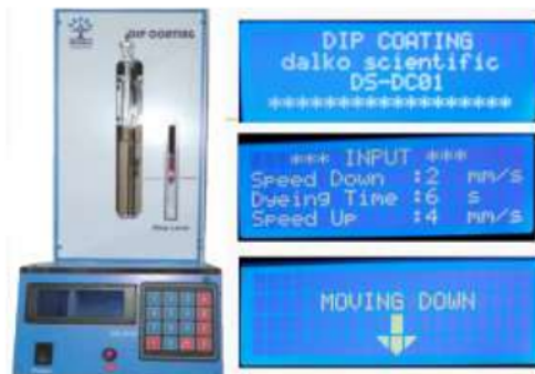
Fig. 5. System (hardware) of dip coater
