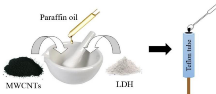
Figure 2. Preparation of the modified electrode (MWCNTs: multiwalled carbon nanotubes, LDH: layered double hydroxide).
