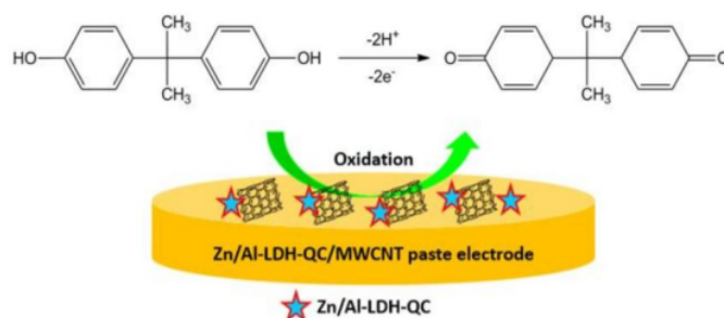
Scheme 1. The electro-oxidation reaction of bisphenol A on electrode surface during electrochemical sensing.
