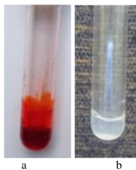
Figure 5. Sample solubility of methyl red in water in oil microemulsion gel in the composition of water (pH 4.5), SDBS, and pentanol. (a) gel before the methyl red dye was dissolved, (b) gel after the methyl red dye was added.
