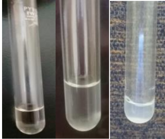
Figure 3. Sample of water in oil microemulsion gelation. a. water in oil microemulsion, b. Water in oil microemulsion sol, c. Water in oil microemulsion gel.
