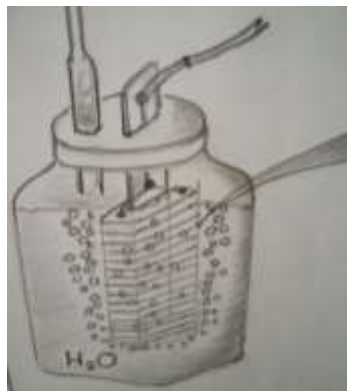
Gambar 1. Skema manual disain elektroda trapping
