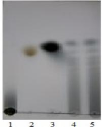
Fig.-7: TLC Chromatogram of Inulin Hydrolysis Product.
