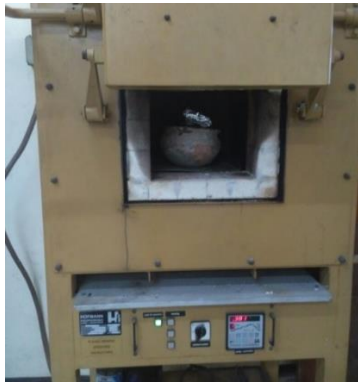
Fig 4. Carbonization Process of Tibarau Sugarcane Briquettes in Furnaces
