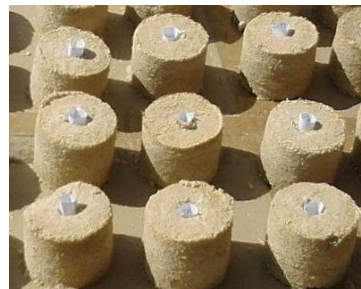
Fig. 6 Tibarau Sugarcane Briquettes Before the Carbonization Process
