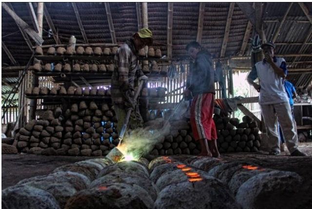
Figure 1: Pouring Brass Liquid into the Mold
