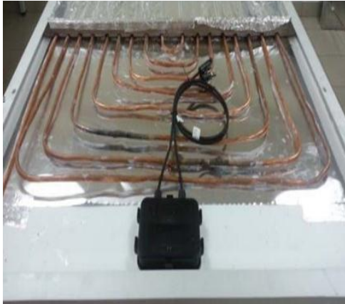
Fig. 2. Copper pipe as water flow conduit
