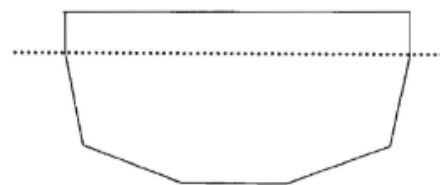
Fig. 1. "Akatsuki" type of hull bottom
