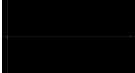
Figure 4: Visualization of the SAR test elements within the program. The vertical line is the azimuth line ( Y -axis), the horizontal line is the range line ( X -axis), the two white bars in the left side are the transmitting antenna and the receiving antenna, the white bar in the right side is the corner reflector (point target). Distance between antenna and the corner reflector is 100 m.
