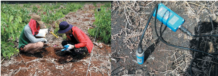
Figure 2. Volumetric soil moisture measurement by the TDR probes.
