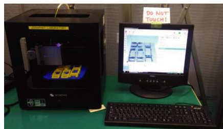
Figure 3: Fabrication of pyramidal X-band horn antenna using 3D printer.
