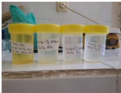
Figure 1. Results of Sol-Gel-varying concentration of Al-Zn dopant from left to right with a concentration of 0 %; 1 %, 5 %, and 10 %.
